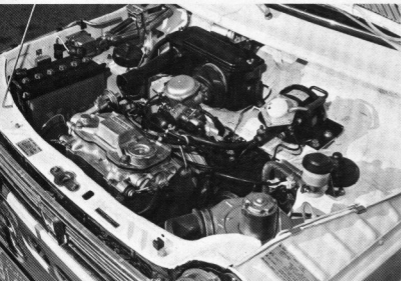
Above: Two-cylinder Honda 600 engine looks a lot like a motorcycle power plant until you discover a differential and cooling fan attached. Top right: As in the Fiat, the Honda's interior is simple and direct. Strange positioning of shift lever does cause problems during gear changes. Right: Trunk space in the Honda is sadly lacking with a smallish cubic/cubic sufficing.
